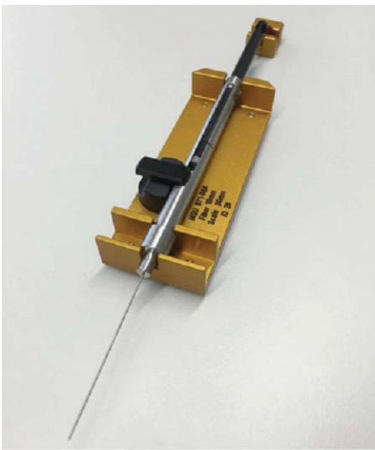
▶ SPME Fiber Holder for CTC auto-sampler
