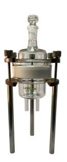
Designed for liquid or gaseous test chemicals and gaseous collection media. Permeation cell NW50 in accordance to EN 16523-1 (replaces EN374-3) for testing PPE films such as safety gloves or safety clothing in order to measure the permeability of the test substances to the samples.
