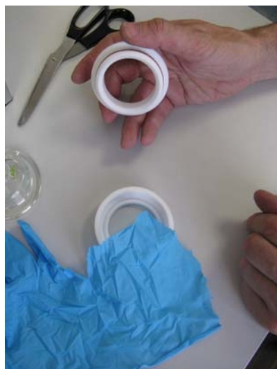
Set the glove sample on the lower part of the PTFE jig.
