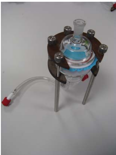
Hand tighten the thumbscrews. Do not use tools, because of breakage.
