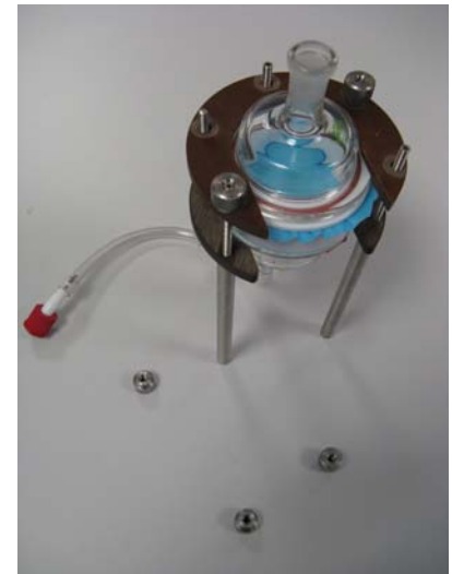
Upper bracket molding compound (groove points down!) hang up and screw crosswise.
