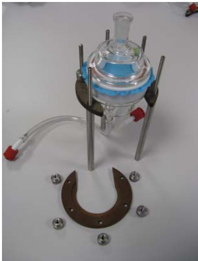
Put on the PTFE-jig and the cap.
