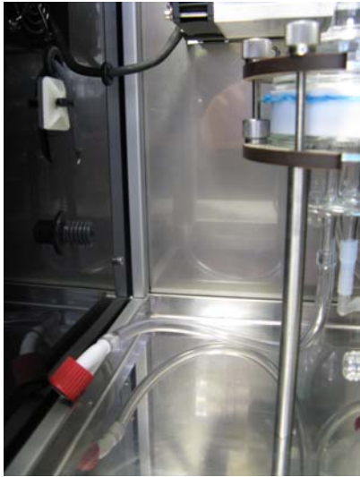
Remove the PTFE-tube from the permeation cell with the air (left!).
