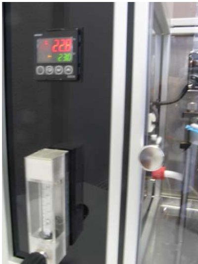
The temperature is automatically called for a test temperature of 23\text{ }^{\circ}\text{C} \pm 1\text{ }^{\circ}\text{C} .
