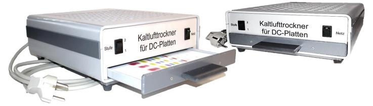
By pull out to the device drawer a TLC record (max. 20 x 20 cm) can be inserted. The drawer is closed again and the net plug is pocketed. The device is put into operation about the green seesaw counter (shines green). About the black step counter the strength of the airflow can be chosen: Step 1: two ventilators / step 2: four ventilators. From above after the introduction the space air is sucked over a fleece filter and the TLC record is dried.
