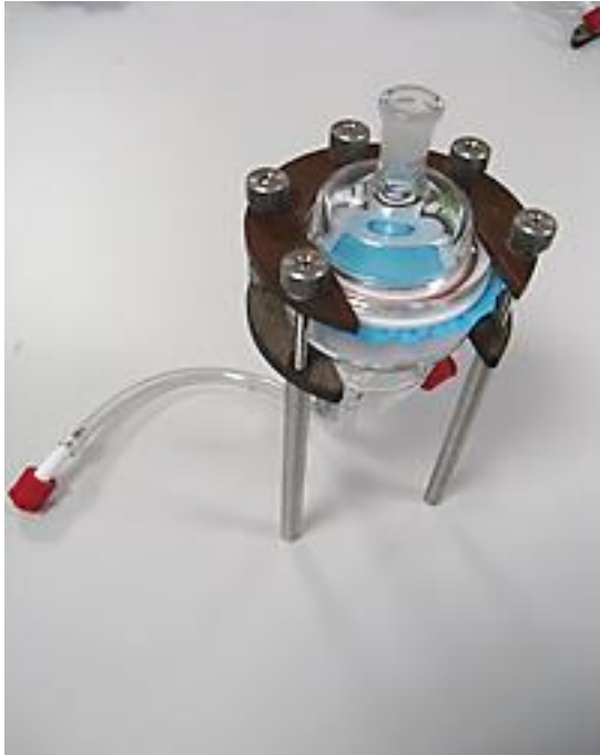
Tighten the knurled screws by hand. Do not use a tool due to the risk of breakage
