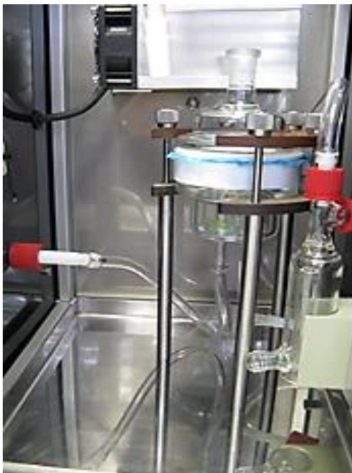
Tightly (by hand) screw the permeation measuring cell's clear, transparent PVC hose to the air inlet (left!).
