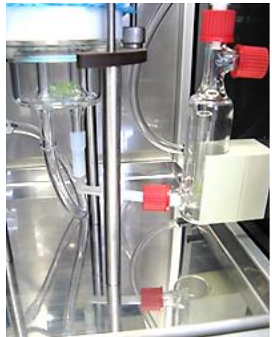
Tightly (by hand) screw the milky PTFE hose to the air equalization tank
