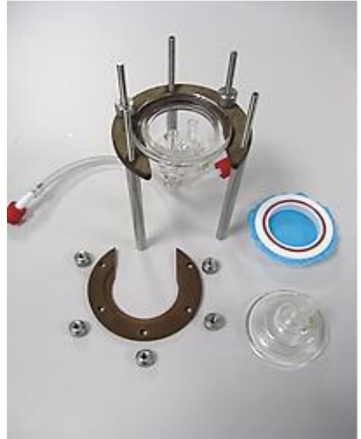
Prepare the permeation measuring cell
