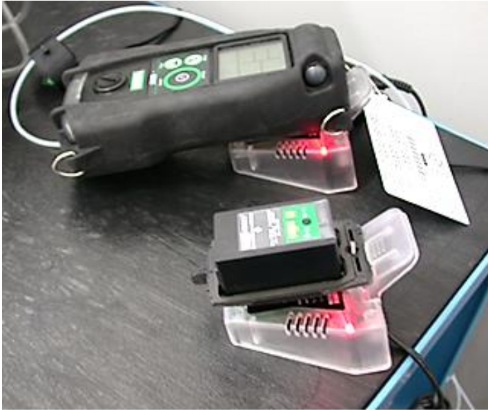
Charge the batteries (Sirius® + flow meter)
