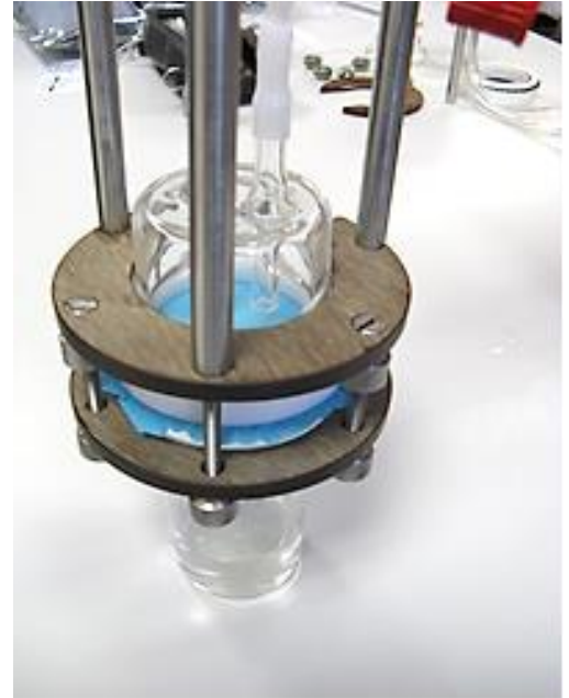
Completely empty the permeation measuring cell
