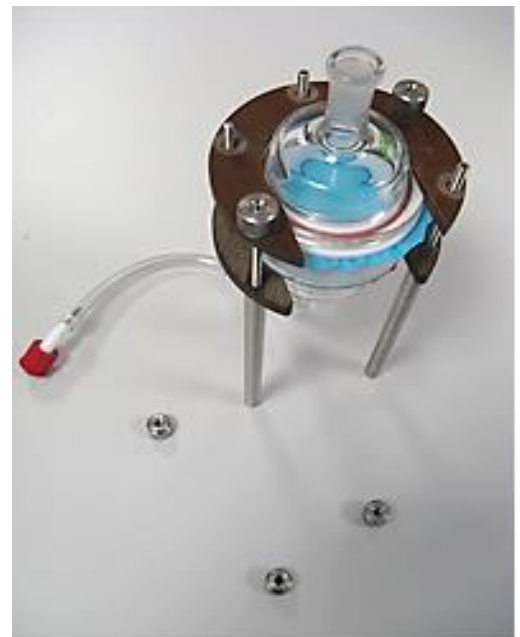
Place on the upper bracket from the moulding material (nut points downwards!) and screw into place with the cross-head screws
