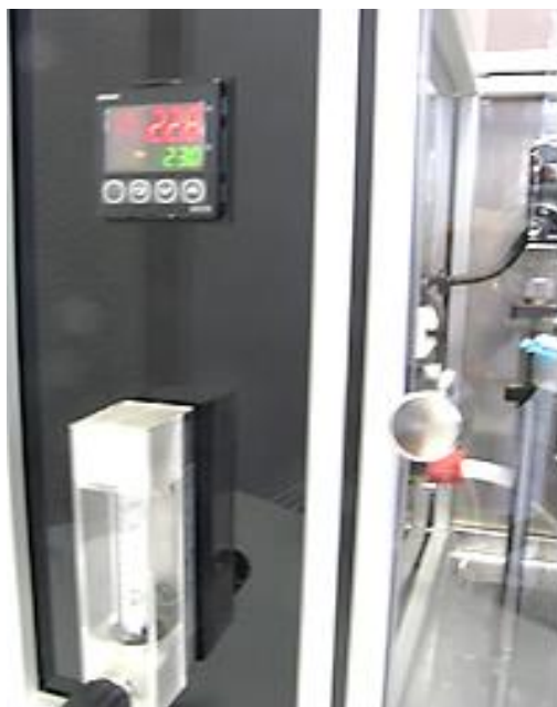
The temperature automatically sets itself to the necessary test temperature of 23\text{ °C} \pm 1\text{ °C}
