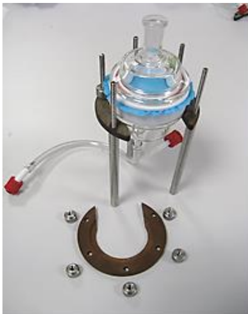
Put the PTFE clamping device and the upper part into place
