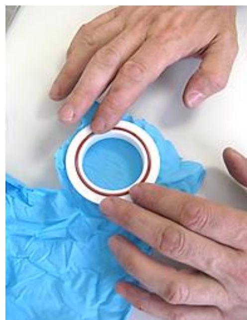
Clamp the protective glove sample into the bracket
