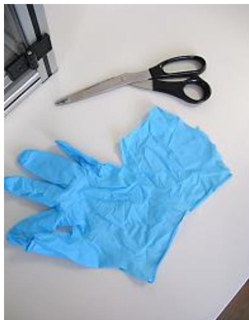
Roughly cut the protective glove sample
