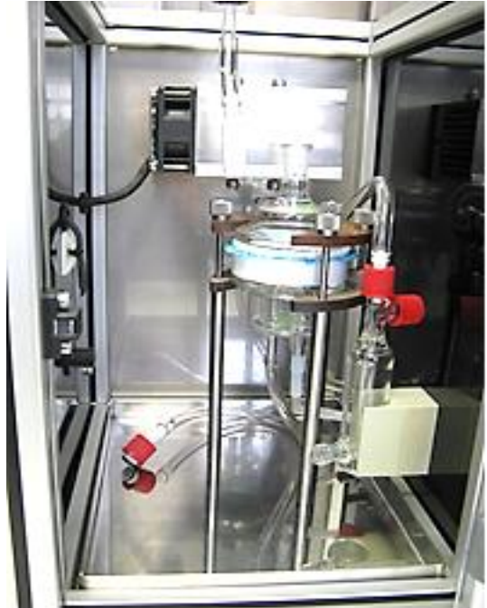
Position the permeation measuring cell at the back right
