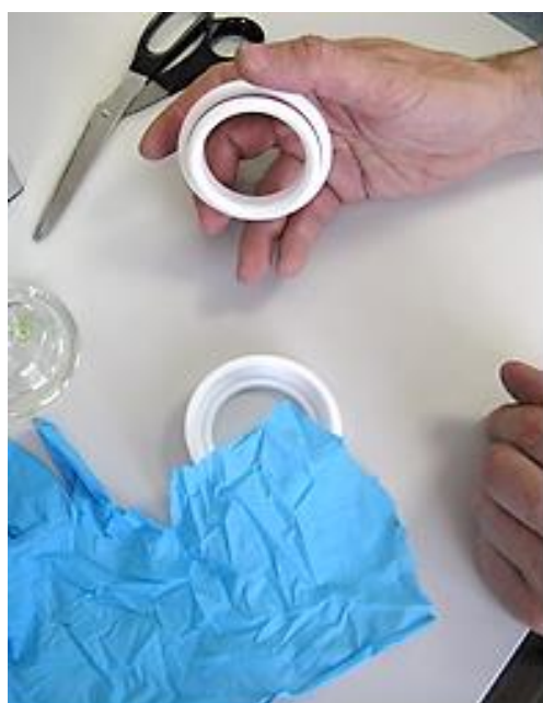
Place the protective glove sample on the lower part of the PTFE clamping device
