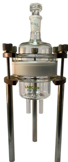
Designed for liquid or gaseous test chemicals and gaseous collection media. Permeation cell NW50 in accordance to EN 16523-1 (replaces EN374-3) for testing PPE films such as safety gloves or safety clothing in order to measure the permeability of the test substances to the samples.
