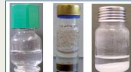
Figure 7. Vials after i) extraction (left, billimex®), ii) centrifugation (middle) and iii) drying (vortexed) with Na<sub>2</sub>SO<sub>4</sub> (right).
